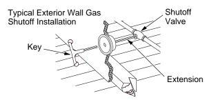
Figure 18 - Manual Shutoff Valve Installation
